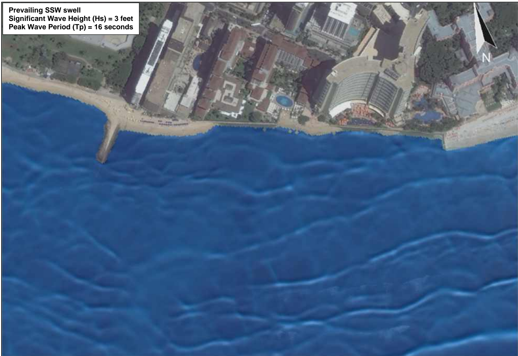
Figure 8-8 XBeach-NH wave pattern for high-prevailing SSW swell – Halekūlani beach sector
