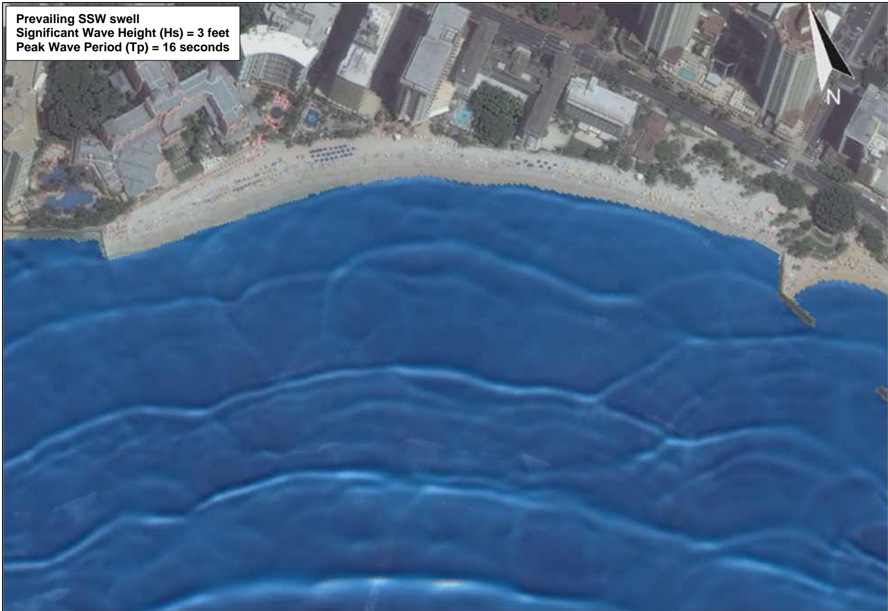
Figure 8-9 XBeach-NH wave pattern for high-prevailing SSW swell – Royal Hawaiian beach sector
