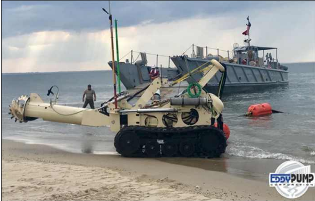
Figure 3-10 Remote Operated Submersible Dredge (Eddy Pump®, 2021)
