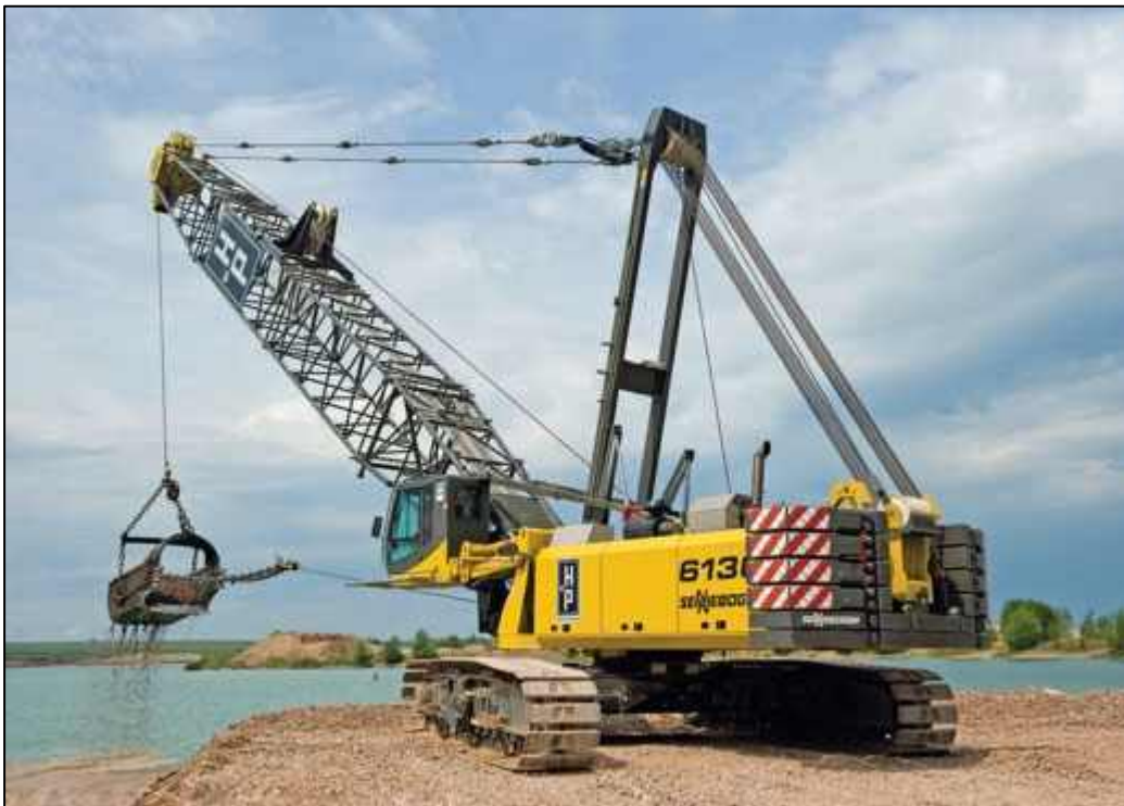
Figure 7-21 Sennebogen 6130 HD duty cycle crawler crane ( www.sennebogen.com )
